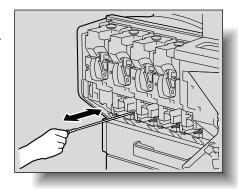
**3** Securely insert each charger-cleaning tool, and then close the front door.
